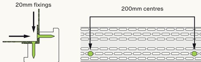
Fig. 8 - Use of perforated closure on corner profiles
