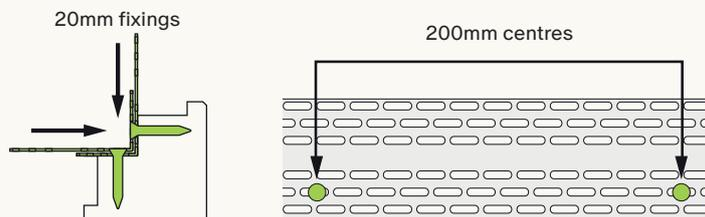
Fig. 8 - Use of perforated closure on corner profiles
