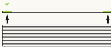
Lift boards on the edges using 2 people to lift at a time
